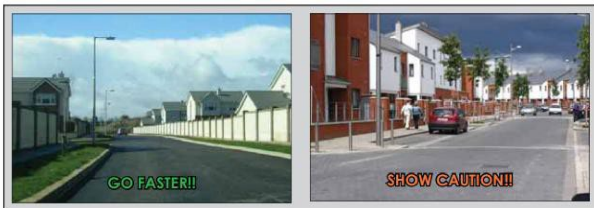
Figure 42: The elimination of access and frontage along roads was introduced to reduce risk, but it serves to encourage speeding (DMURS, 2013)
