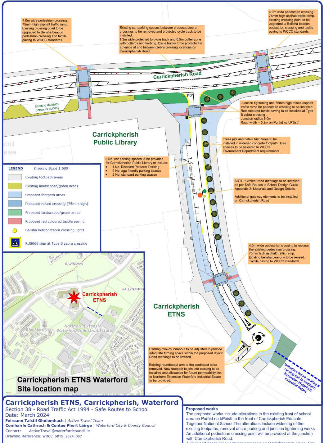
This proposed layout is for information only and is subject to change at the detailed design stage. This drawing is copyright of Waterford City & County Council and is for information only. Unauthorised printing, copying, sending or projecting of this drawing is prohibited.
