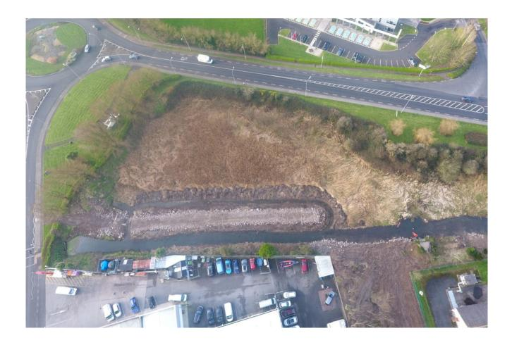
A new safe access was installed at the head wall on the pond adjacent to Aldi carpark to facilitate removal of litter that accumulates at this location. This access will facilitate more regular cleaning of this area.
